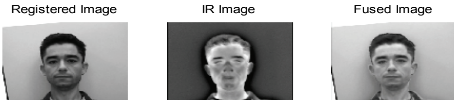
Fig. 4. The Result of Fusion: Left: Registered Images, Middle: IR Image Right: Fused Image with GA.
